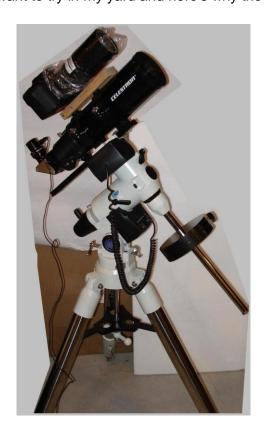
The piggyback mount is a piece of scrap oak that I drilled three holes in and used three ½" bolts I already had. I didn't even have to cut the wood. That's fast!
