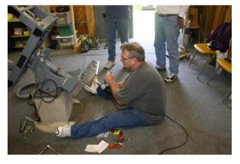
Once we are happy, the two remaining holes are drilled in the plate and angles and the bolts are inserted and tightened.
