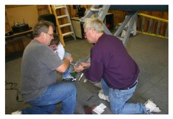
Next, the drive is placed on the coupling so that the fit can be judged.
