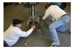
Once the polar shaft was bare of the old drive, we – I'll just mention one more time that Howard and Craig did most of the physical work – cleaned up the shaft and tried the adapter. It only fit part way up, with rough spots on the shaft causing binding. After scrounging for some time, we found a piece of Emory cloth in the block house, probably used in the observatory painting project, and managed to clean up the shaft sufficiently to mount the adapter.
