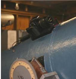
The images above show the "piggy back" bracket for the 20"scope. The bracket allows the camera to be mounted at various positions. The image on the left shows the camera mounted at the end of the tube (left) and the image on the right shows a position closer to the center.
